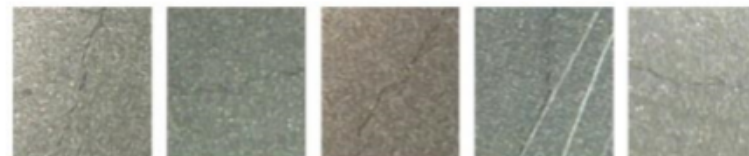
(a) Tiny cracks with low contrast and different brightness.
